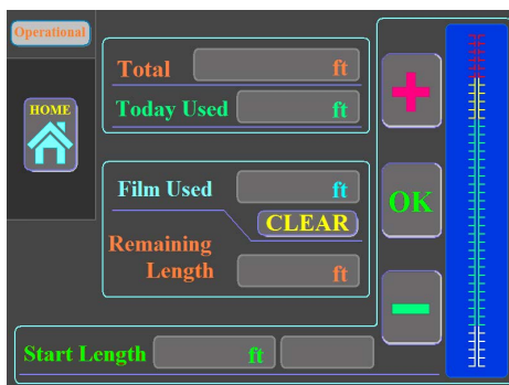
FILM USAGE COUNTER Tracks the film usage per job, per day, and lifetime.
