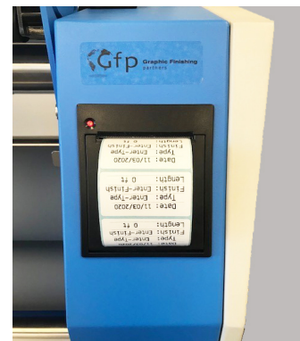
ROLL LABEL PRINTER generates pressure sensitive label with film description and remaining footage for labeling partial film rolls.
